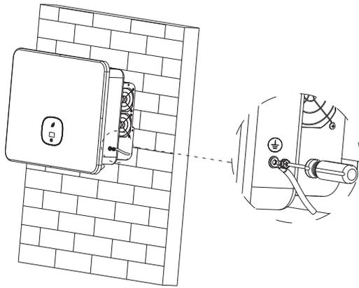
Fig 6.1 Grounding diagram
